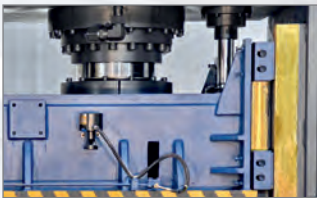
Adjustable 8 points Self-Lubricated (Graphite impregnated bronze material) Oil less Guide ways
