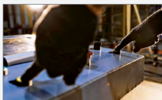
Two-hand operator safety to ensure accident-free operation
