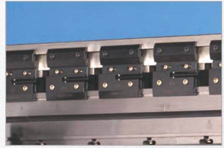
Quick Release Clamp with taper wedges for localized bending degree adjustment
