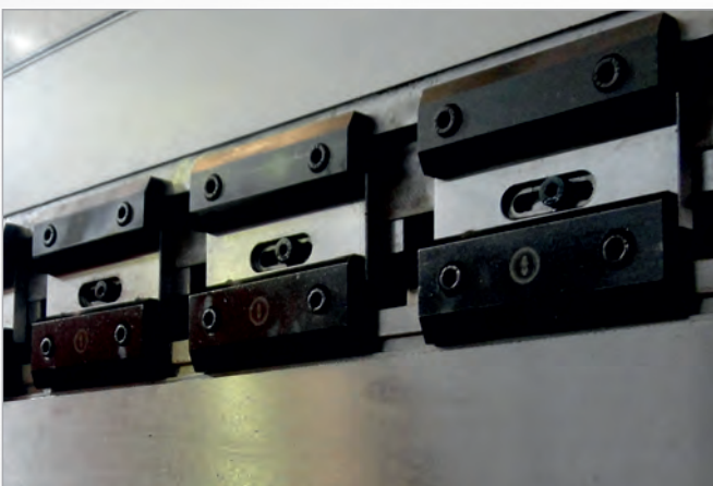
Allen Type Clamps with Tapper wedges for localized bending degree adjustment.
