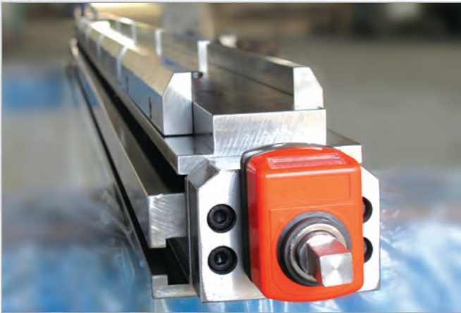
Manual Crowning to get the accurate angle in centre of the machine
